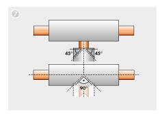
In the case of  $90^{\circ}$  T-joints, the pipe insulation for the branch line should be cut to a point with two  $45^{\circ}$  angled cuts, starting from the centreline.
