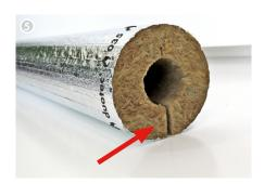
To minimize heat loss when installing horizontally, align the longitudinal seam so that it is at the bottom of the pipel  $^{11}$
