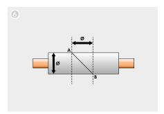
For **90° bends**, cut the shell at a 45° angle as described below – ensuring that the longitudinal seam is positioned at the top. Mark two parallel lines in the middle of the shell, spaced according to the outer diameter of the insulation. Then cut the pipe shell diagonally from point A to point B.
